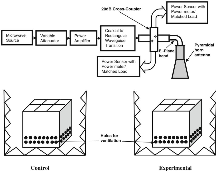
**Fig. 1** Diagrammatic representation of the microwave exposure setup and the position of animal cages during microwave exposure. Mice were exposed to 2.45 GHz low-level MW radiation for 2 h/day continuously for 45 days by using microwave source and pyramidal horn antenna
